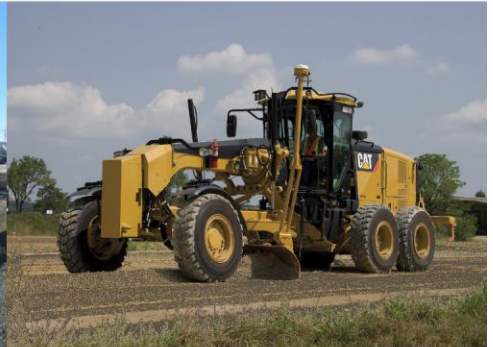
3. RESHAPE MATERIAL TO NEW ROAD PROFILE
